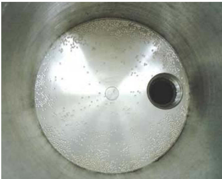
Penn State researchers filled a cylindrical bucket with glass beads and measured the force needed to put an object into motion.
