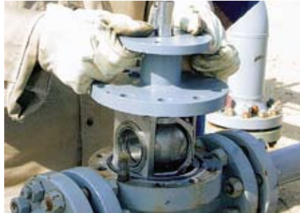
FIG. 3 New cartridge valve combines benefits of a quarter-turn valve with durability of a gate valve.
